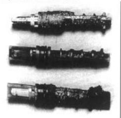
Inspecting the orifice tube on OT systems can provide an important warning before you retrofit. The severe sludging, metal wear particles and, in the top OT some desiccant particles, can alert you to the danger of a bare-bones retrofit.
